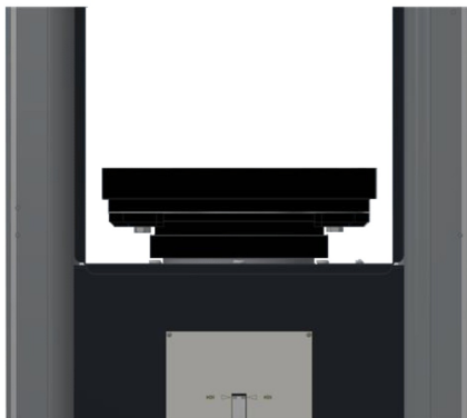
Bottom compression platen of the compression machine/frame fixed by 2 steel plates model 50-C9080/F (side view)
